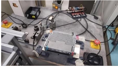
Figure 8 - Screwing load cells
